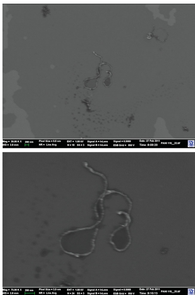
Figure 4. HRSEM images of PANI-coated Nanocyl 7000 MWNT, polymerized in toluene, two magnifications. [Color figure can be viewed in the online issue, which is available at wileyonlinelibrary.com .]
